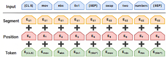
Figure 2: Illustration of the multi-layered process used by the CodeBERT model to transform individual tokens into embeddings via various layers.
