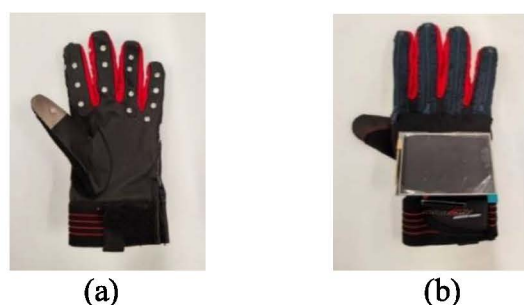
Fig. 1. The prototypes of the left-hand message-sending glove (a) and the right-hand message-receiving glove (b)
