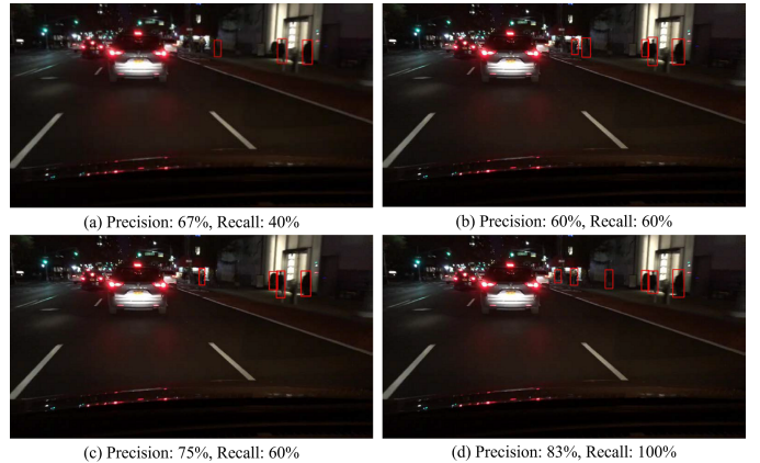
Fig. 1. Advance object detection techniques such as (a) RetinaNet [18], (b) YOLOv3 [16], and (c) SFT-Net [19], exhibit demonstrable limitations in accurately identifying the 'Person' class under low luminance conditions. In contrast, our proposed approach (d) showcases a superior capacity for accurate detection under these challenging light conditions.
