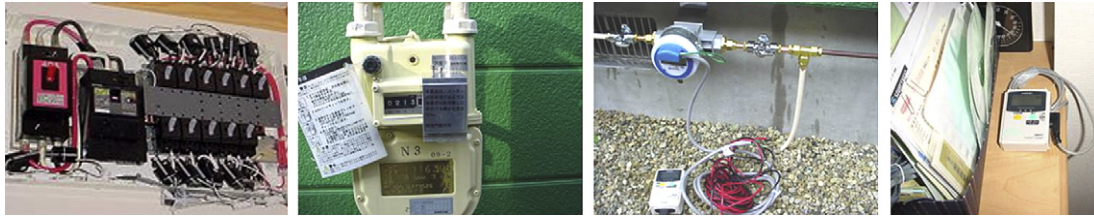
Fig. 6. Measuring instruments (from left to right: electricity, gas, kerosene and air temperature).
